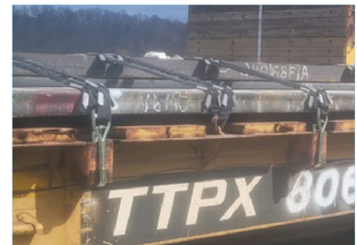
Example of acceptable J-Hook placement on outside face due to car deck design
