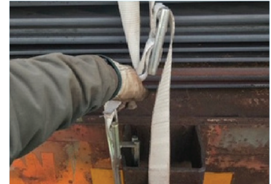
J-Hook has rotated during transit, losing tension and creating problematic loads
