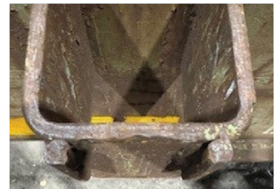
Example of a stake pocket that requires the JHook to be placed on right or left side
