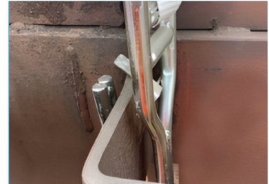
Updated J-Hook placement The strapping anchor is on the interior of the stake pocket, oriented to the left or right face
