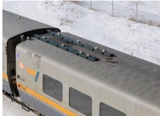
Figure 2.3 Configuration des antennes de VIA Rail
